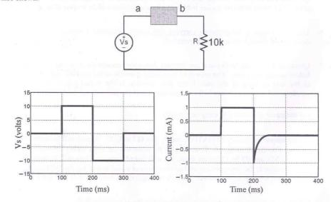
The element connected between  $\mathbf{a}$  and  $\mathbf{b}$  could be
